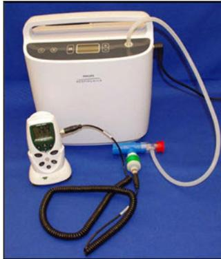
3. Allow the device to continue running the automated “Learn Pressure Bal” test. This portion of the test will take approximately 80 minutes. The unit will shut down when this portion of the test is complete.
