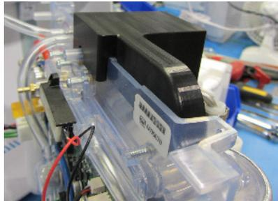
9. Loosen the outlet tube using two wrenches and then allow the metal tube to sit in the jig.
