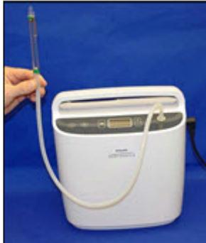
21. Holding the flowmeter in the vertical position above the SimplyFlo, observe the flowmeter scale and record the reading on the Test results sheet
