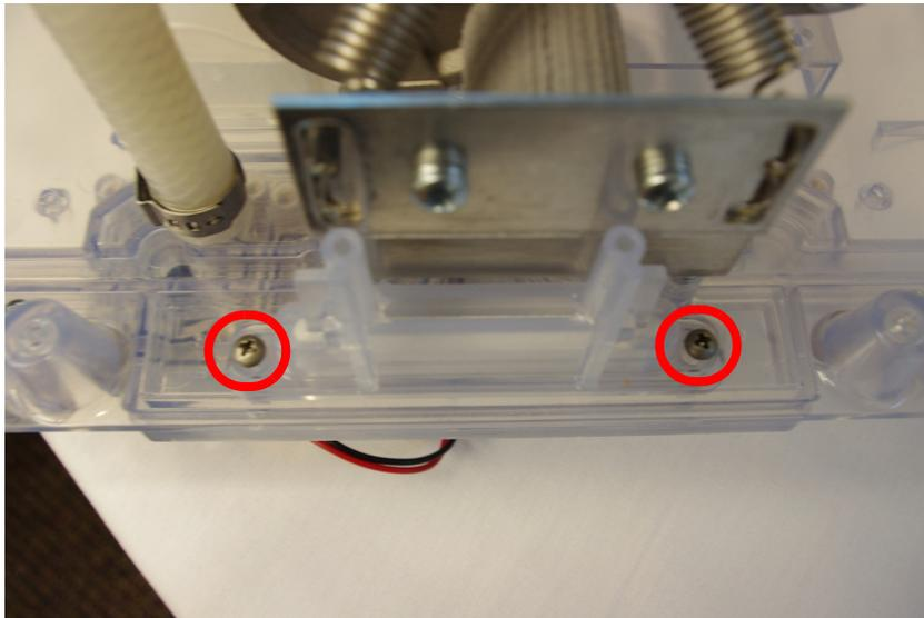
5. Remove the Exhaust Muffler and the Gasket.
