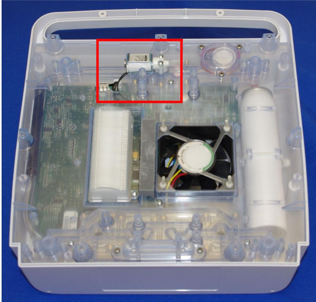
4. Remove the two screws that secure the Sieve Bed Balance Valve to the spine assembly.
