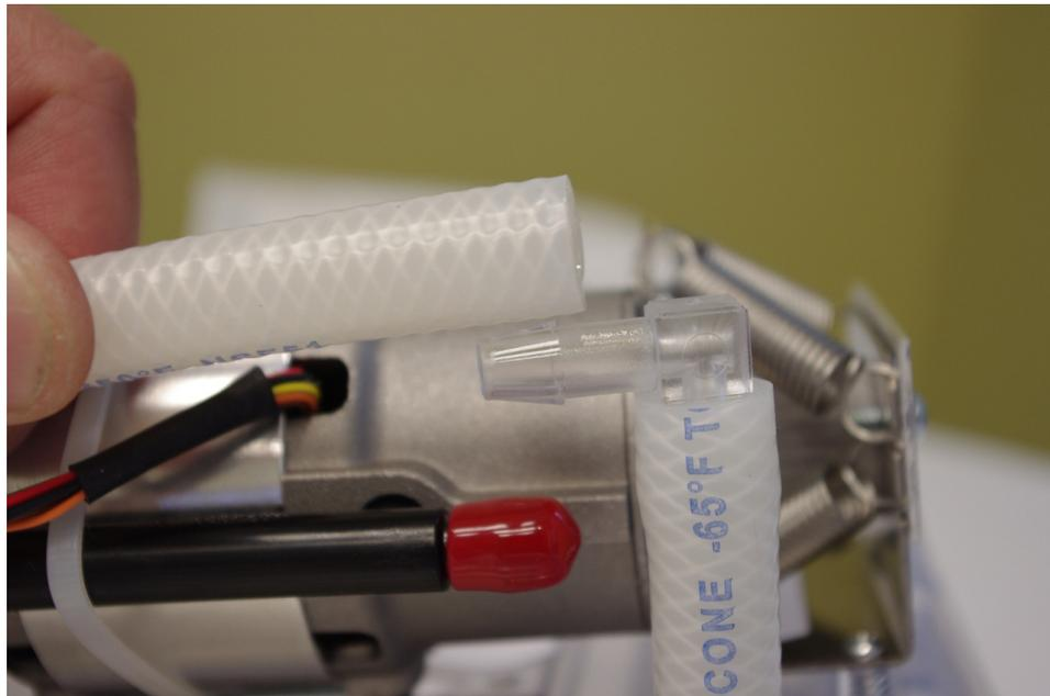
7. Remove the intake hose from the Compressor intake manifold.
