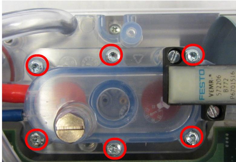
3. Remove the Check Valve and Gaskets from the spine assembly.
