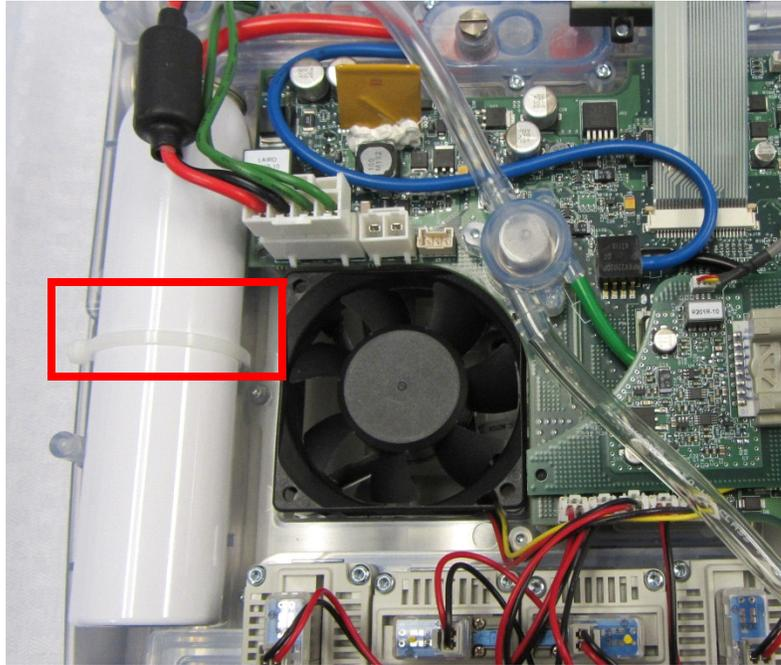
3. Disconnect the product tank tube from the Check Valve housing.
