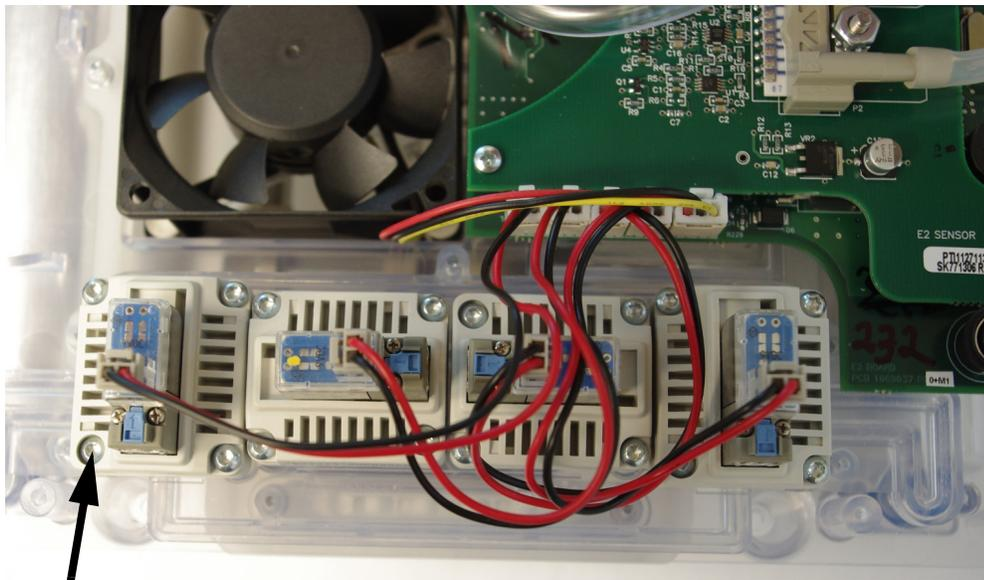
3. Remove the four T10 Torx screws securing the valve(s) to the spine assembly.
