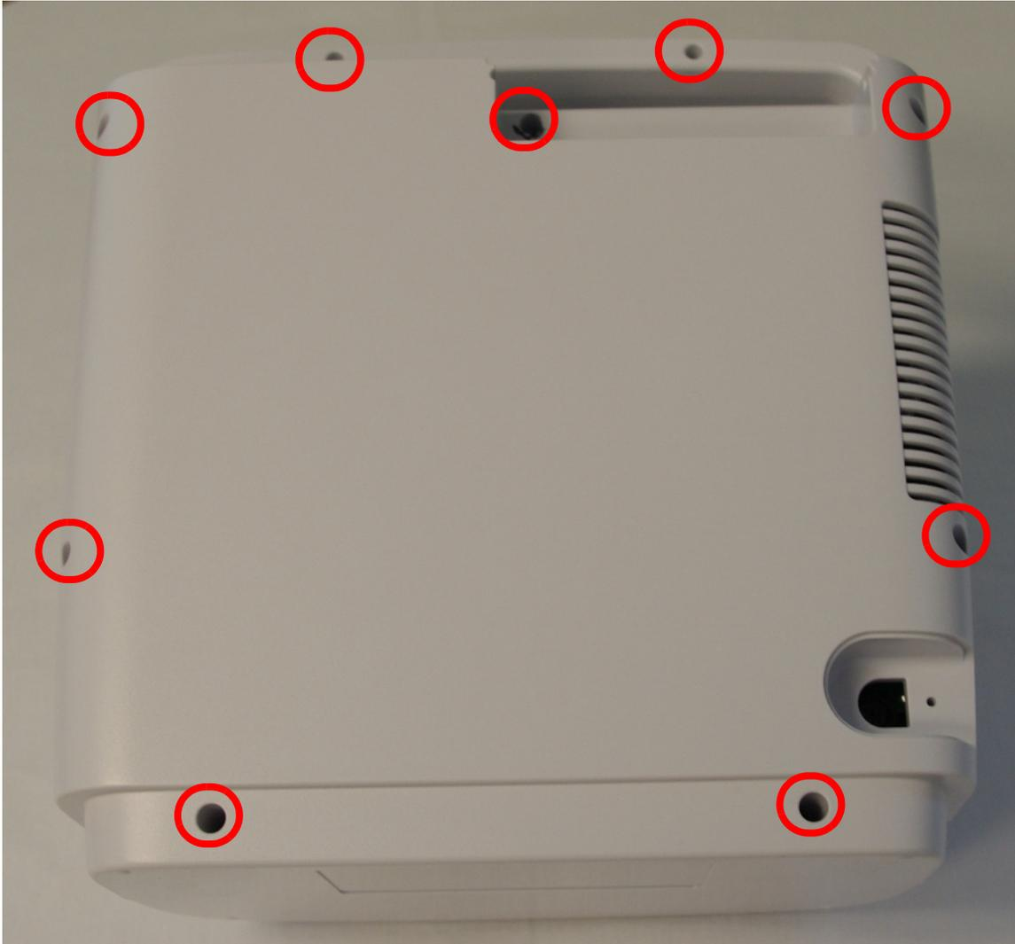
3. Adjust the device so the handle is facing you and the battery compartment is facing up.
