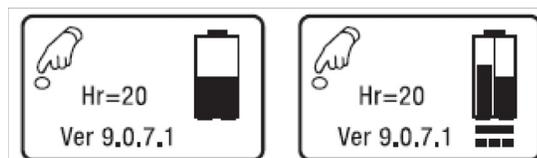
3. Press the Power button a second time to place the device in operating mode. This second press helps prevent unwanted starts or inadvertent changes in oxygen flow. The introductory screen momentarily appears, shown at the left below, followed by the final operating mode screen, shown at right.
