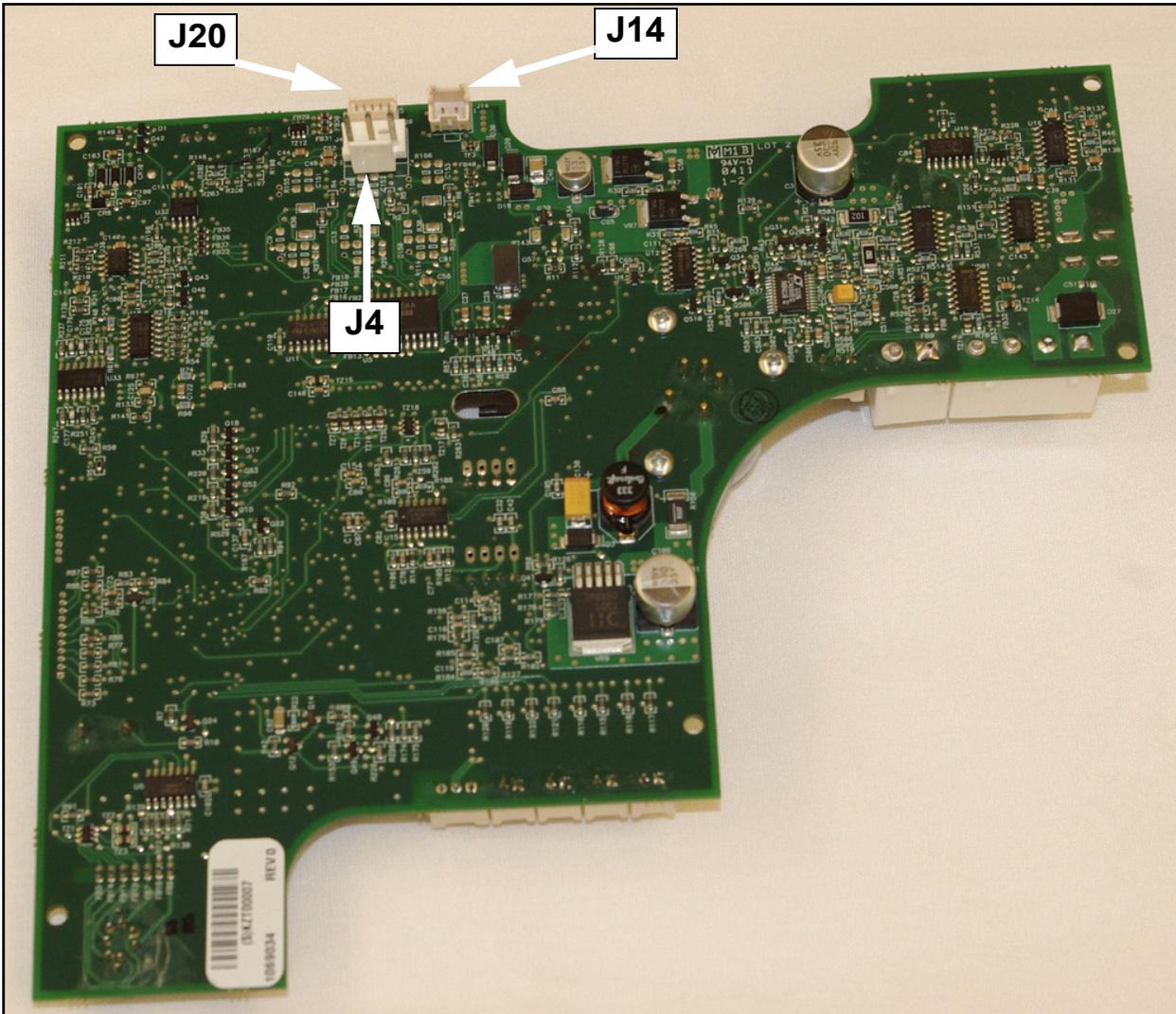
FIGURE 7-1 REAR SIDE CONNECTIONS
