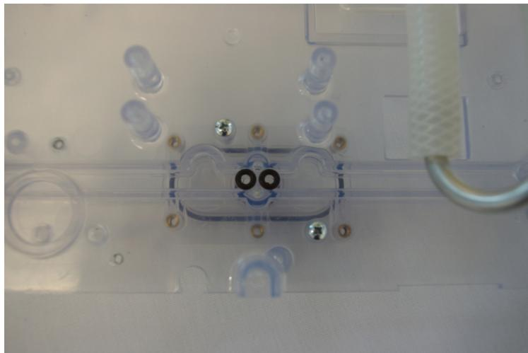
2. Install the Sieve Bed Balance Valve with wire harness towards the opening in the spine assembly.
