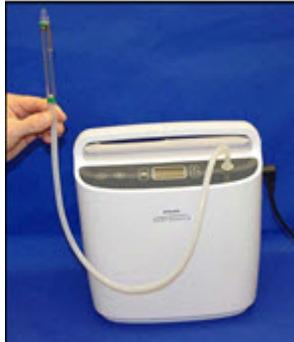
36. Holding the Flowmeter in the vertical position above the SimplyGo, observe the Flowmeter scale and record the reading on the Test results sheet.
