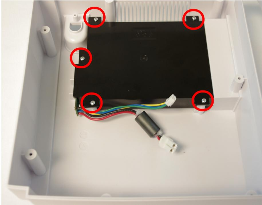
3. Remove the Battery PCA from the Battery Enclosure.
