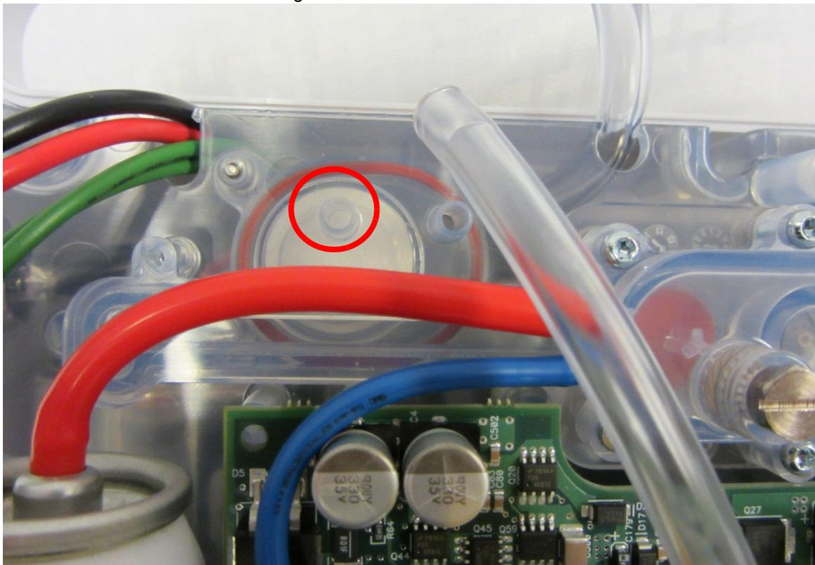
6. Remove the 7 screws securing the Spine Assembly to the Front Enclosure and remove the Front Enclosure.
