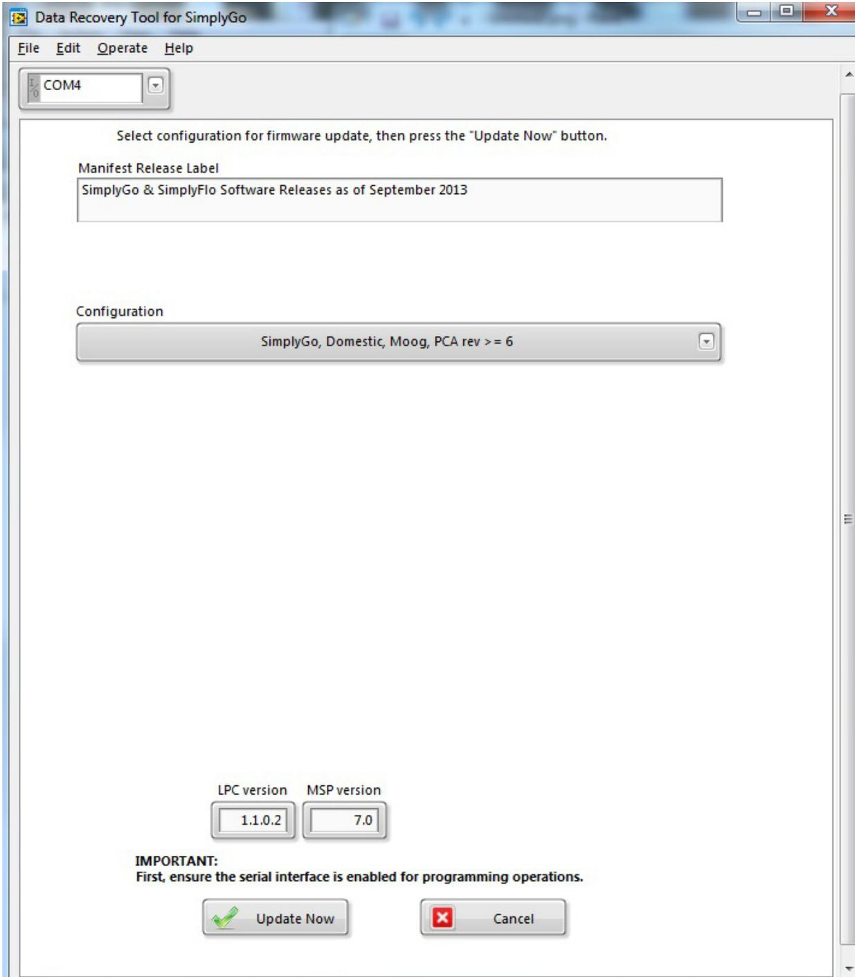
18. Once the device has completed the code load and rebooted proceed to step 19.
