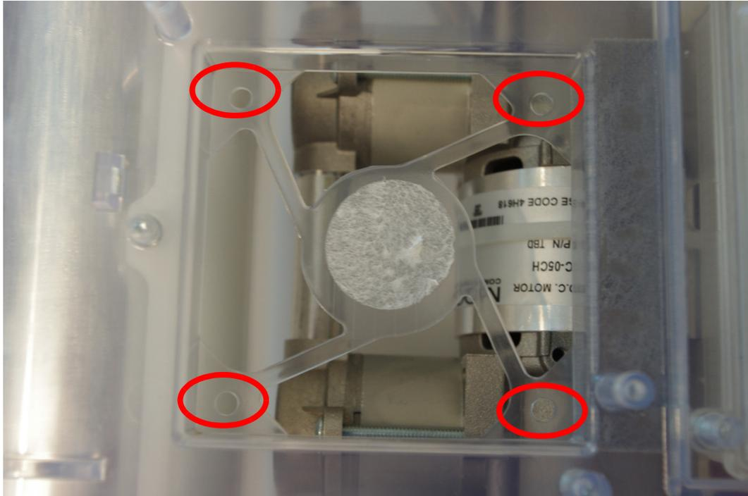
2. Push the rubber mounts completely through the holes in the spine assembly to lock the fan assembly in place. If the rubber mounts do not go through the holes grab the rubber mounts with your finger and pull until it is completely through the hole.
