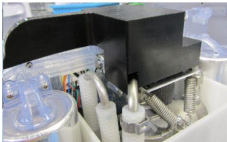
10. Tighten the clamp to finish the connection at the other end of the metal outlet tube.
