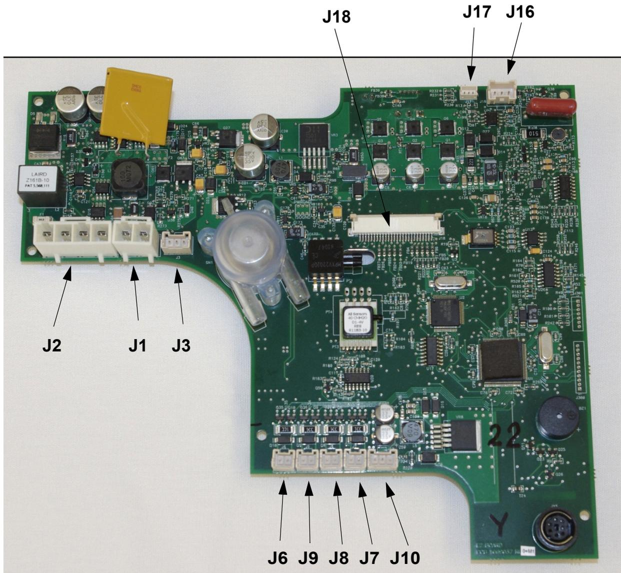
FIGURE 7-2: FRONT SIDE MAIN PCA CONNECTIONS
