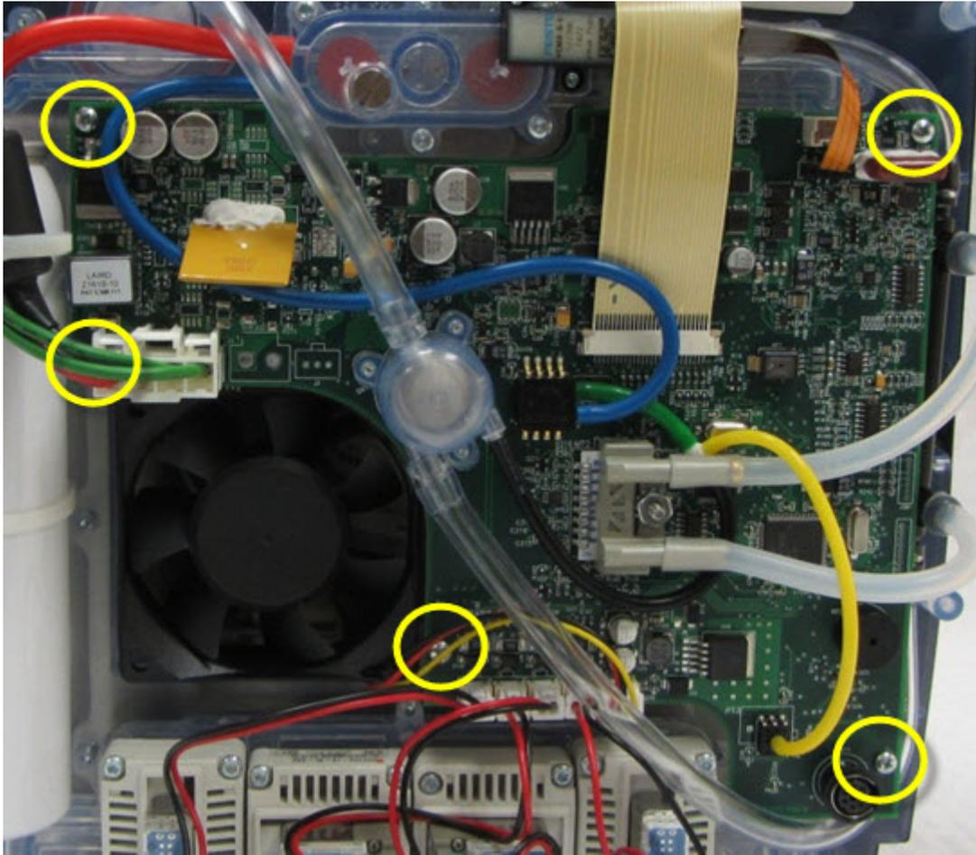
10. Disconnect the Sieve Bed Balance Valve from J14 on the Main PCA. This connection can be found on the rear side of the Main PCA.
