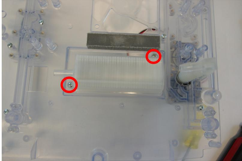
8. Remove the Inlet filter from the Spine.
